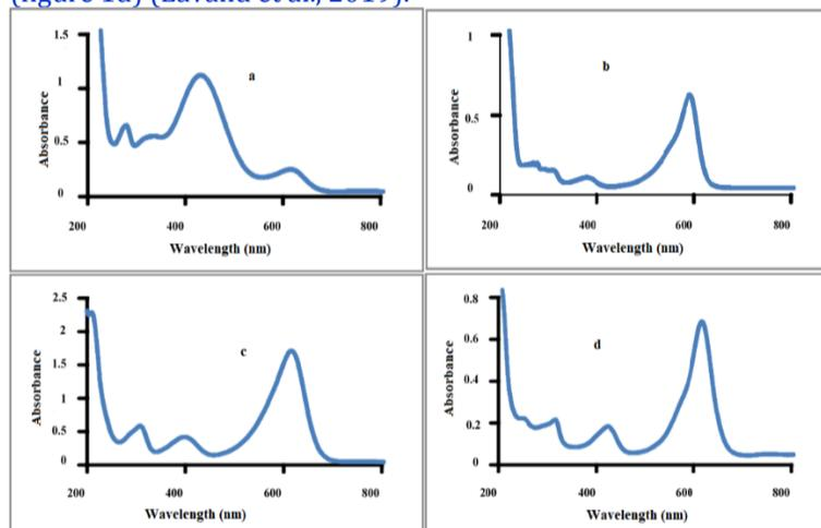
Figure 1: UV- visible spectrum of Bromothymol blue(a), Bromophenol blue(b), bromocresol green(c), malachite green(d).
